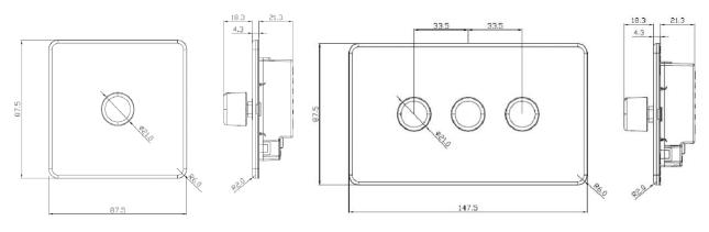
Push on/push off control. Advanced trailing edge type dimmer suitable for dimming all types of lamps both resistive and inductive. Minimum capacity: 5W dimmable LED or 10W incandescent. Maximum capacity: 150W dimmable LED or 200W incandescent. Suitable for mains lighting, low voltage lighting and LED lighting (for compatibility please check with lamp manufacturer.
