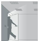
**Absence Detection:** Upon entering the room the person switches on the light as normal, when no movement is detected the detector switches off the lighting automatically. Lights can also be switched off manually.
