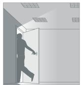
**Presence Detection:** Detectors will switch on lighting automatically when a person enters the room, and switch off lighting automatically when no movement is detected.
